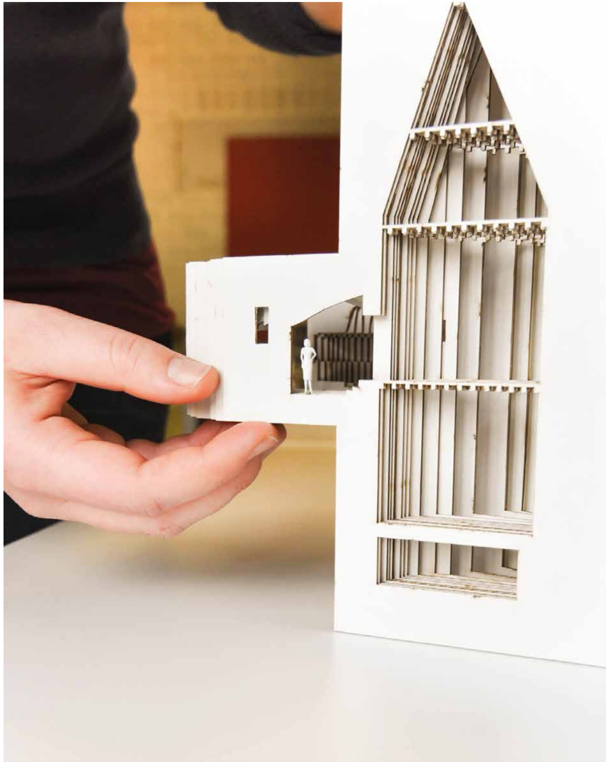
[11] book made out of laser-cut sections investigates the smallest wing of Gruuthuse palace
