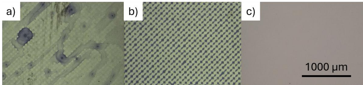
Figure 3: Optical microscopy images (Keyence) of PEDOT:PSS coatings deposited from aqueous solution, illustrating the effect of mesh release timing. (a) Too early : film still wet, causing droplet formation and inhomogeneous coating . (b) Too late : film fully dried against mesh, leaving a periodic thickness imprint of the screen relief. (c) Optimal timing: homogeneous, featureless coating (scale bar: 1000 \mu\text{m} ).
