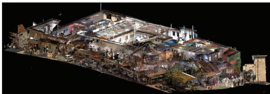
Fig.5: The point-cloud 3D model of Pilavoglu Han Model is prepared by the laser scanning data in FaroScene by the Project Team.
